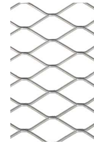
Large mesh 1 L 60.0 mm W 32.0 mm B 3.0 mm A 1.5 mm F 0 81.3 %
