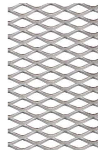
Medium-sized mesh 3 L 30.0 mm W 15.0 mm B 4.0 mm A 1.5 mm F 0 46.3 %
